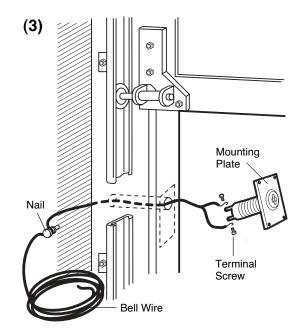
**Step 4:** If screw nails won't hold the plate firmly in place, use anchor and nut supplied with hardware. (See illustration on page 2). If anchor and nut are used, remove the Key Switch terminal screws.
