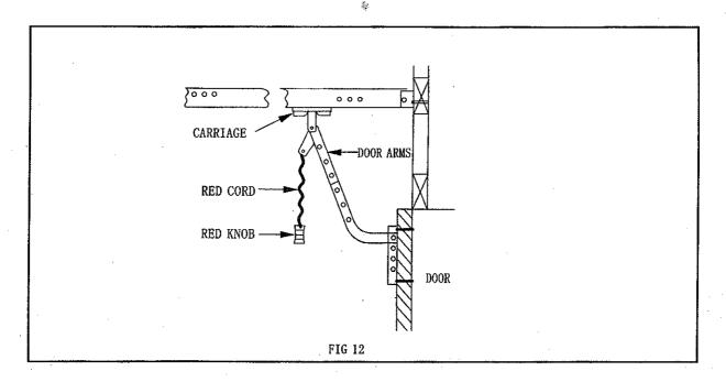
To reengage carriage to drive mechanism, pull the red cord down and toward the door. When power is reactivated, press push button to automatically reconnect the carriage to the drive mechanism. You can also manually raise or lower the door to engage the drive mechanism.
