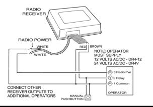
**DESCRIPTION** The Delta-3 DR4V & DR4-12 digital receivers are four-channel wireless radio controls designed for use with automatic garage/gate operators and access control systems. The receivers can be activated by any of the Delta-3 format transmitters. **Receivers must be mounted at least 8 feet apart.** The Delta-3 radio format provides 256 different digital codes. The codes are set using the 8-position coding switches in the units.
