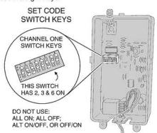
STEP 2B GRD-2 Channel 2 code setting. Select any valid combination of ON and OFF positions for each of the switch kevs numbered 1 - 8. Use a different code combination than that used for channel one switch.
