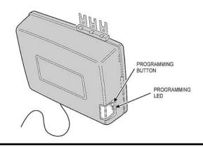
**STEP 5** Program receiver. Momentarily press the receiver's program button. The red programming LED will light if there's room in the receiver's memory for another transmitter (40 maximum per receiver). The LED stays on for about 5 seconds. A transmitter must be entered while the LED is on. Press the desired transmitter button. The LED will flicker indicating that the receiver has accepted the transmitter.
