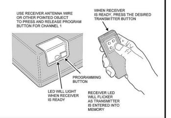
**STEP 6** Add additional transmitters. Repeat Step 5 for each transmitter used with this receiver. Be sure to press the receiver's program button *each time* a new transmitter or a different transmitter button on a multi-button transmitter is pressed. If the LED doesn't come on when the receiver's program button is pressed, the receiver's memory is full (40 transmitters total). Use the erase function (Info 1) to remove transmitters from the receiver's memory.
