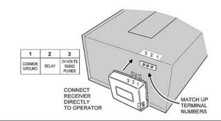
STEP 1B MDRG Installation (For non 24V Operator). A Model TF524 step-down transformer must be used to power the
