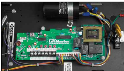
Includes the Medium-Duty Logic Board with Built-In Receiver
