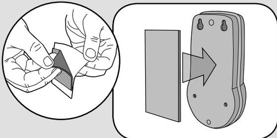
Peel off white paper from mounting tape. Firmly press mounting tape on back of intercom.
