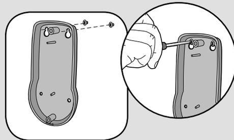
Mount Intercom with small silver screws. Screw the top two screws halfway into the mounting surface. Place back of intercom over screws. Tighten screws.
