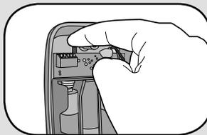
Press the Learn button on the new intercom until a beep is heard. Within 10 seconds put any networked intercom into Learn Mode (refer to table below).
