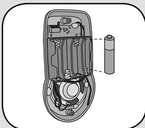
Install 4 AA Alkaline batteries (not provided). (Lithium batteries recommended for colder environments.)
