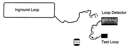
The same test loop can be used for testing loop detectors returned from the field as faulty units.
