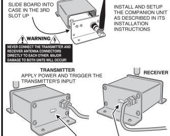
THE RECEIVER'S SIGNAL INDICATOR SHOULD LIGHT AND **OUTPUT SHOULD ACTIVATE**
